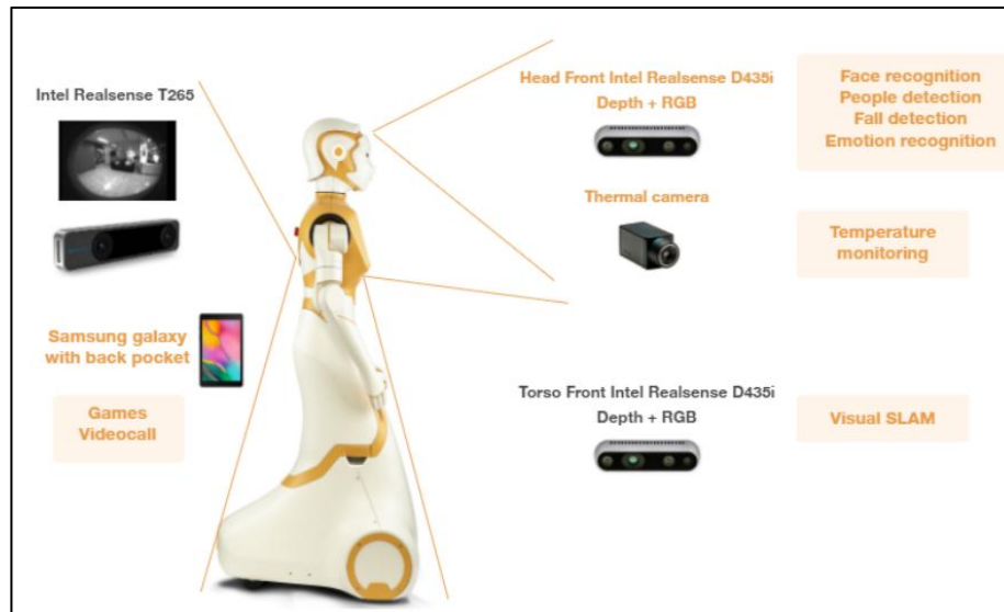
Figure 158 - Component Architecture of PT1-UC004 and Hardware Components to be used
