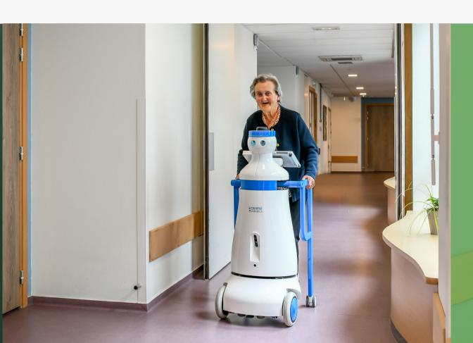
Kompaï-3 EHPAD developed by KOMPAÏ Robotics (France) is equipped with walking assistance bars for physical tasks and was designed to assist people with reduced functionality and capabilities and their caregivers.
