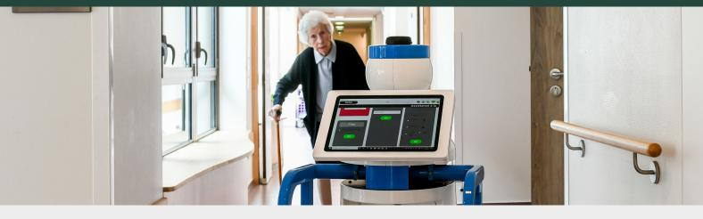
**Kompaï-3 EHPAD robot** version, developed by **KOMPAÏ Robotics**, was designed to assist people with reduced functionality and capabilities and their caregivers. With the basic **Kompaï-3 EHPAD** version, the following function are proposed: mobility assistance for residents; tours (information, entertainment, night surveillance, etc.); individual or collective distractions; and logistical capacities within the establishment, such as laundry or waste.
